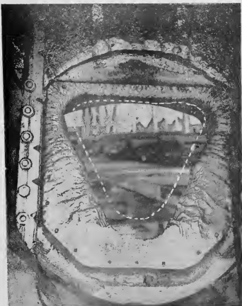
The metal plate above one corner cut from the plates of a sphere which had been magnetized to find out if it was in need of repair. The electrical examination showed that there were cracks somewhere in the welded joints between the plates, and three sample cores were cut out to discover how big and also where they were. The cores show the cracks running through the weld metal.
